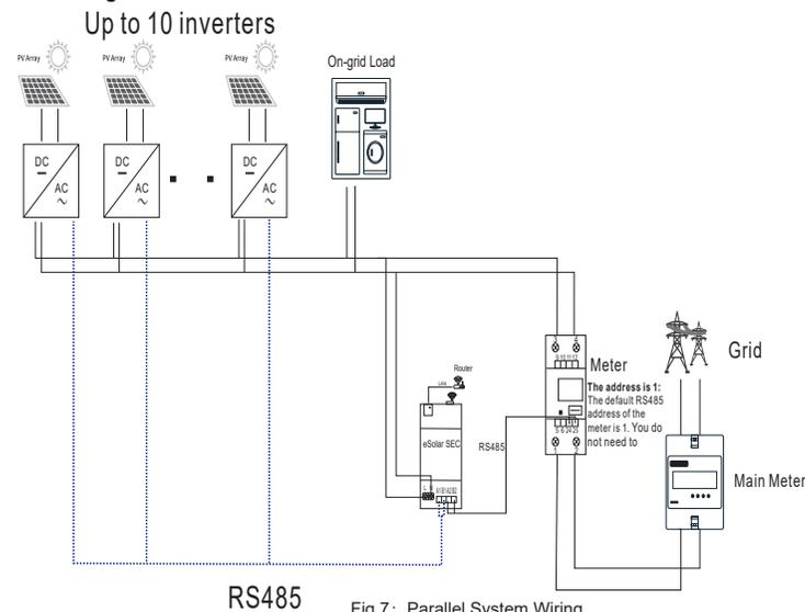
Fig 7: Parallel System Wiring
