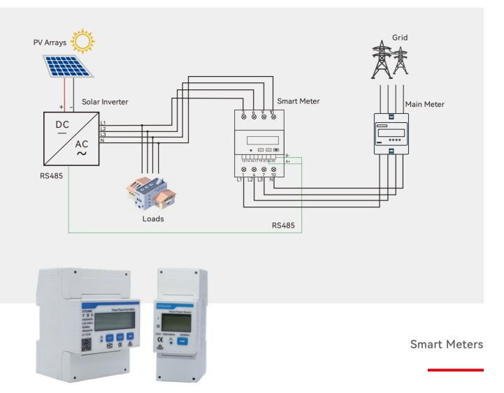
Zero export solution aims to prevent solar systems from exporting excess power into the grid, to ensure the quality and waveform of voltage subject to standards of local authorities. SAJ provides zero export solution to meet emerging technical requirements and various applications on sites. Smart meter measures and calculates the system electrical parameters and interacts with inverter for energy management and zero export control purposes.
