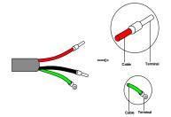
2. Insert the cables through the conduit and connect it to the battery terminals in the wiring compartment.
