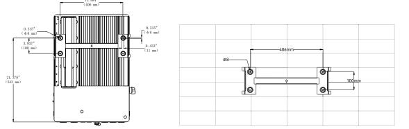
3. Mount the inverter to the plate. Install three M5 screws on each side of the inverter.
