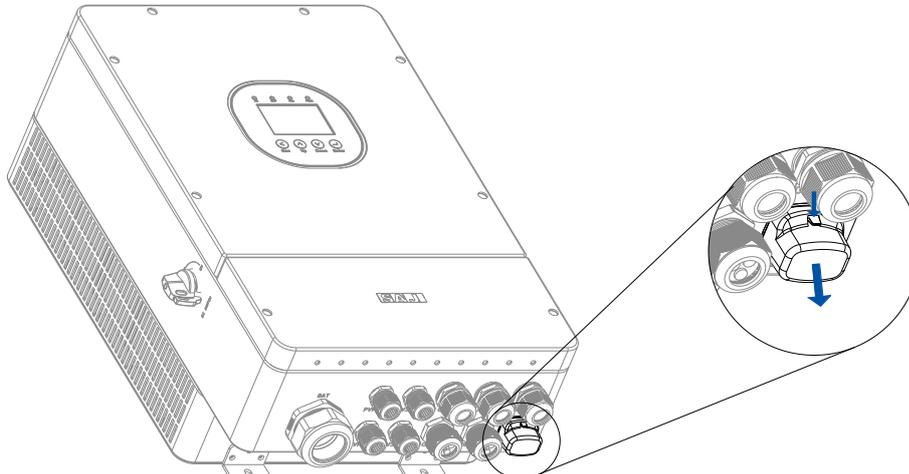
b. Insert the communication module to the 4G/WIFI port and secure the module by rotating the nut.
