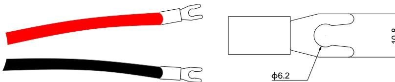
3. Insert the cables through the cable glands GEN, LOAD, and GRID and connect the cables to the corresponding L and N terminals. Then, use a standard torque to tighten the screws on the terminals to secure the cable connection.
