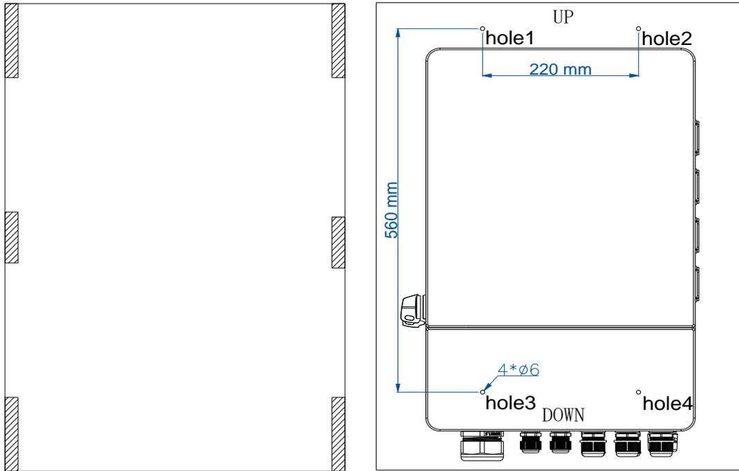
2. Use a rubber mallet to insert four expansion tubes into the holes. Insert four M6\*50 expansion bolts into the drilled holes. Reserve 5 mm distance between the wall and the head of the screw.
