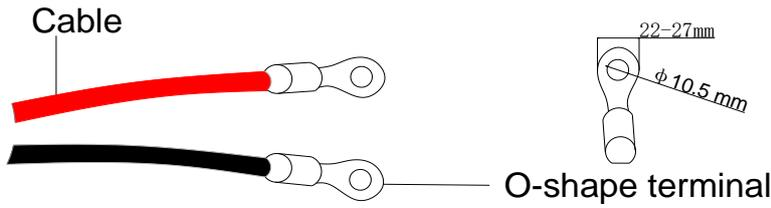
2. Insert the cables through the cable gland BAT and connect the cables to the battery terminals BAT+ and BAT- in the junction box.
