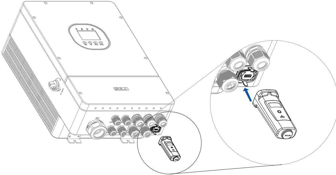
2. (Optional) Connect the battery temperature sensor.
