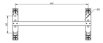
2. Drill Holes and Place the Expansion Tubes. Drill 4 holes in the wall, and then place expansion tubes in the holes using a rubber mallet.
