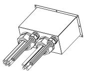
2. Connect the communication cable to the corresponding port. GRID,GEN and Back-up Fix the cables according to conductor marks of L1,L2,L3,N and PE.
