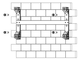
4. Mount the Inverter. Carefully mount the inverter into the rear panel as shown. Make sure that the rear part of the equipment is closely mounted into the rear panel.
